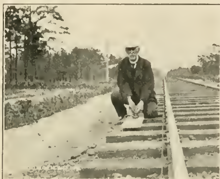
BREAKING THE CIRCUIT To get the exact time on the chronograph of the stop of the train which has just passed.
